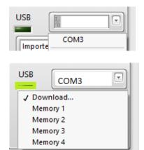
Once the PERMEA3 connected to the computer and on, define the port com which should be used.
